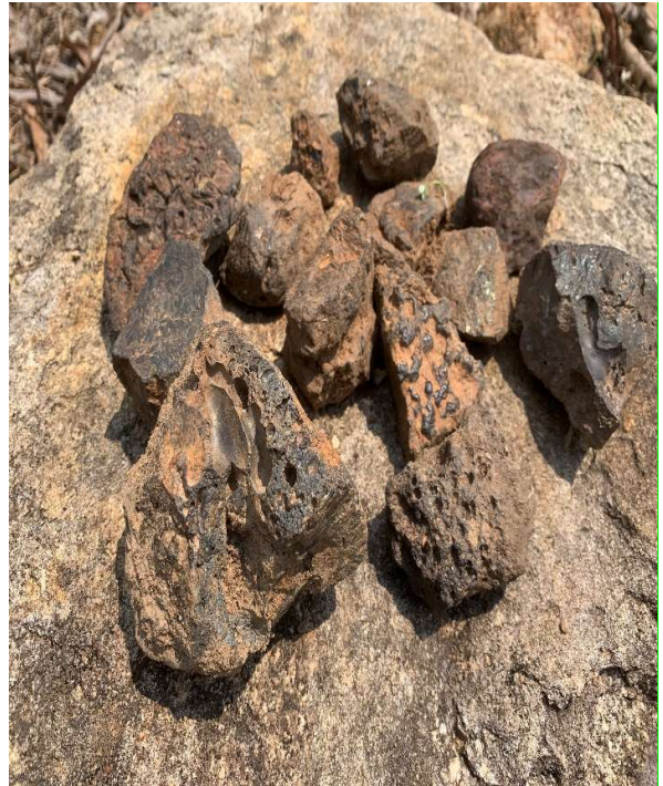
The site of historic iron extraction shows no remains of the furnace, but iron slag, locally known as 'Kittada Kallu' (iron smelting furnace waste), can still be found.
