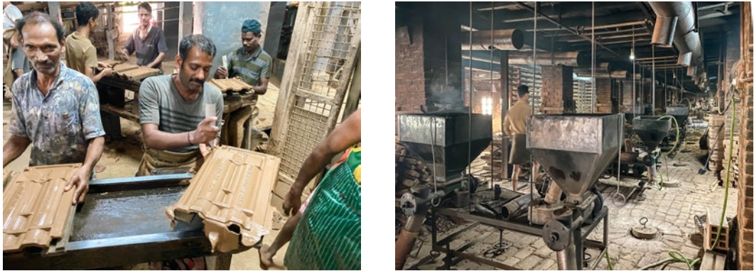
From the left: 1. Scraping excess clay after molding; 2. Cashew nut shells used as fuel for the kiln
