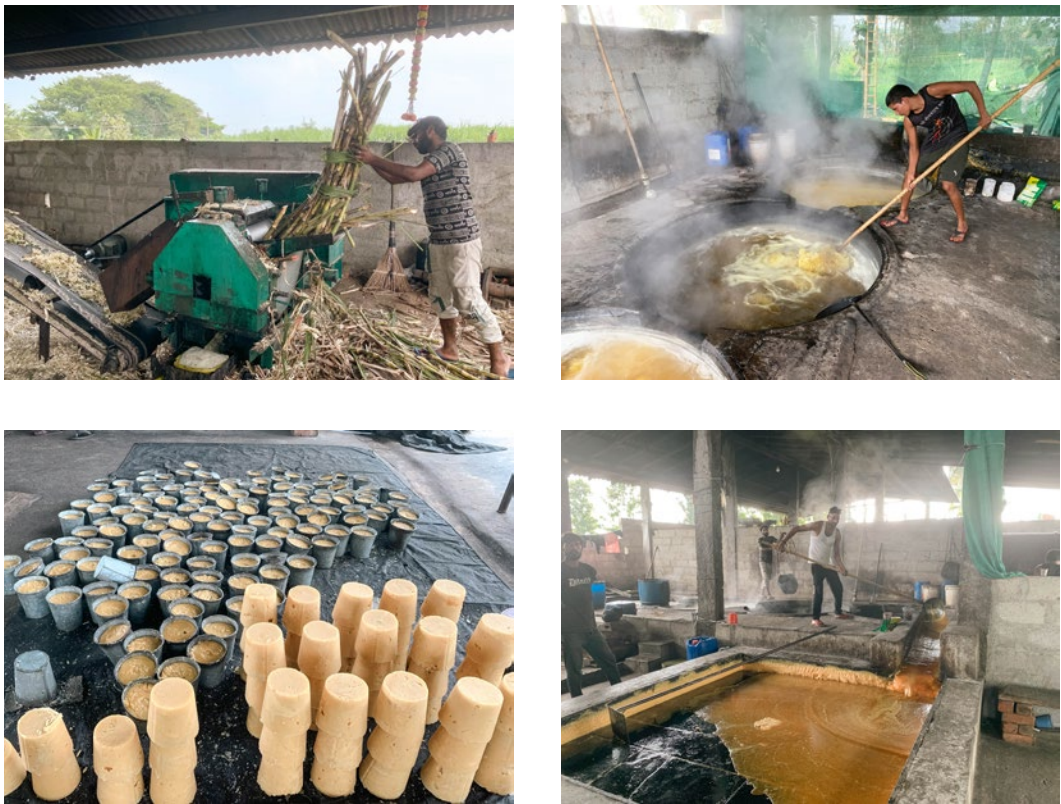
Clockwise from top left: 1. A labourer feeding sugarcane into the juice extractor; 2. A laborer in the jaggery boiling house; 3. Thick jaggery syrup spreading for cooling and solidification; 4. Jaggery from the mold, ready for sale
