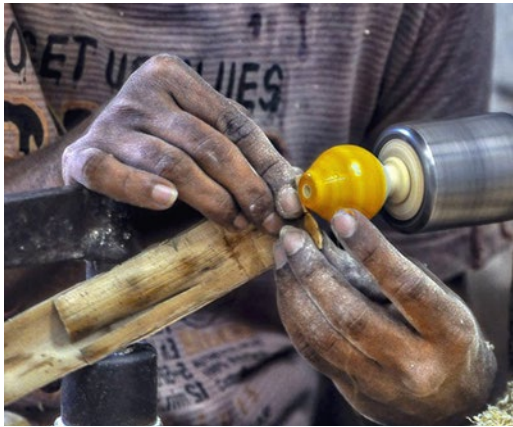
From the left: 1. Lacquering in process during wood-turning operation; 2. Lacquer sourced primarily from Madhya Pradesh
