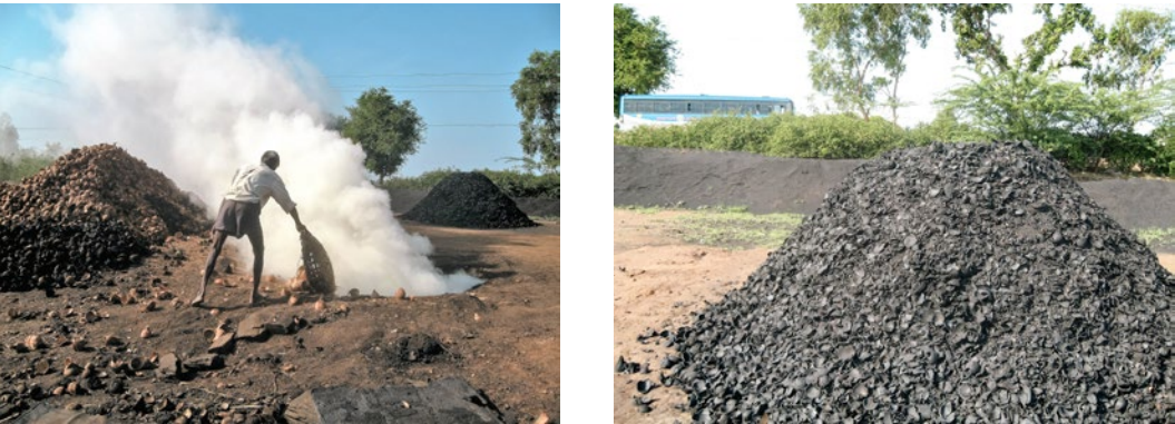
From the left: 1. Charcoals being thrown into the pit; 2. Finished coconut charcoal
