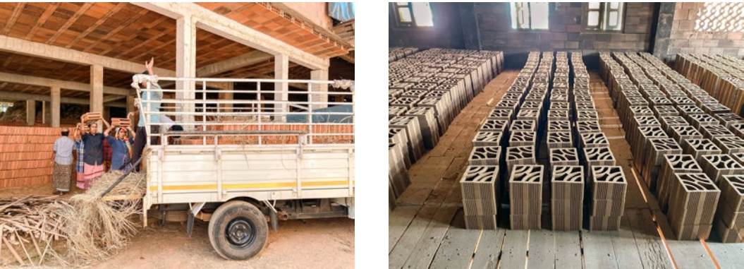
From the left: 1. Molded tiles set for drying before kiln firing; 2. Finished tiles being transported
