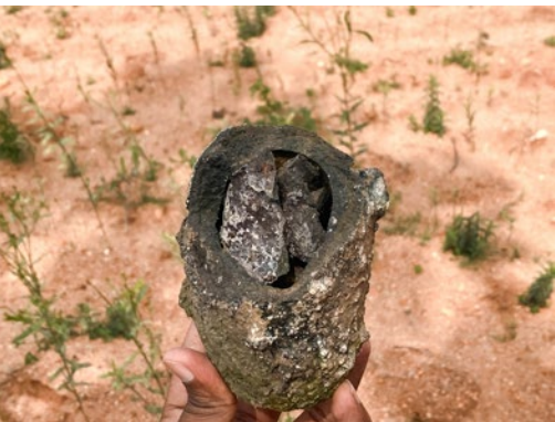
Clockwise from the top left: 1. A shepherd in Maranayakanahalli leads the way to past smelting remains; 2. A crucible and other smelting artifacts found in the steel production area; 3. Debris containing crucibles, tuyeres, and slag remains at the smelting site; 4. The crucible steel-making process: combining iron wedges, Cassia Auriculata leaves, and water in unbaked clay crucibles.
