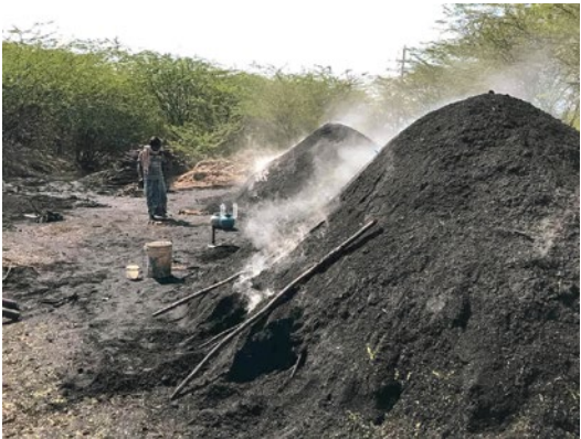
From the left: 1. A laborer cutting large raw limestone into small pieces for kiln charging; 2. Charcoal is prepared nearby as fuel for the kiln. Limestone kilns are still in operation for quicklime production, used for domestic and agricultural purposes. These images were captured at Dodderi near Chalakere as a representation.
