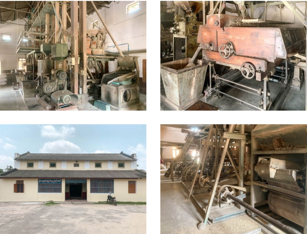
An old huller-type rice mill, Mahadeshwara Swamy Rice Mill at Piriapatna, is still in operation
