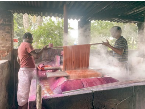
Clockwise from the top left: 1 & 2. At Dommasandra, Bangalore, members of the Devanga community are engaged in synthetic colour dyeing for silk, using various shades. The process involves large vats, with labourers squeezing the silk threads to achieve the desired colour; 3. The plant supervisor inspecting incoming silk threads from customers before processing, currently using artificial dyeing methods; 4. Labourers at the dyeing vat evenly dipping silk threads in the vat
