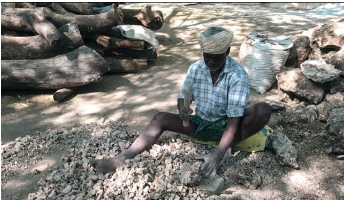
From the left: 1. A laborer cutting large raw limestone into small pieces for kiln charging; 2. Charcoal is prepared nearby as fuel for the kiln. Limestone kilns are still in operation for quicklime production, used for domestic and agricultural purposes. These images were captured at Dodderi near Chalakere as a representation.
