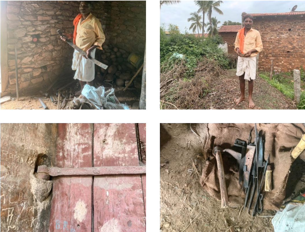
Clockwise from the top left: 1. A man showcasing a slag piece from the era when their ancestors practiced forging and iron smelting; 2. Currently, they purchase raw materials such as iron flat bars and other metal supplies from nearby hardware shops for forging purposes; 3. Blacksmith forging small quantities of agricultural tools such as sickles, tongs, and axes; 4. A metal bar from the Bangalore Fort gate, showcasing a rudimentary native forging style (image for representation purposes)
